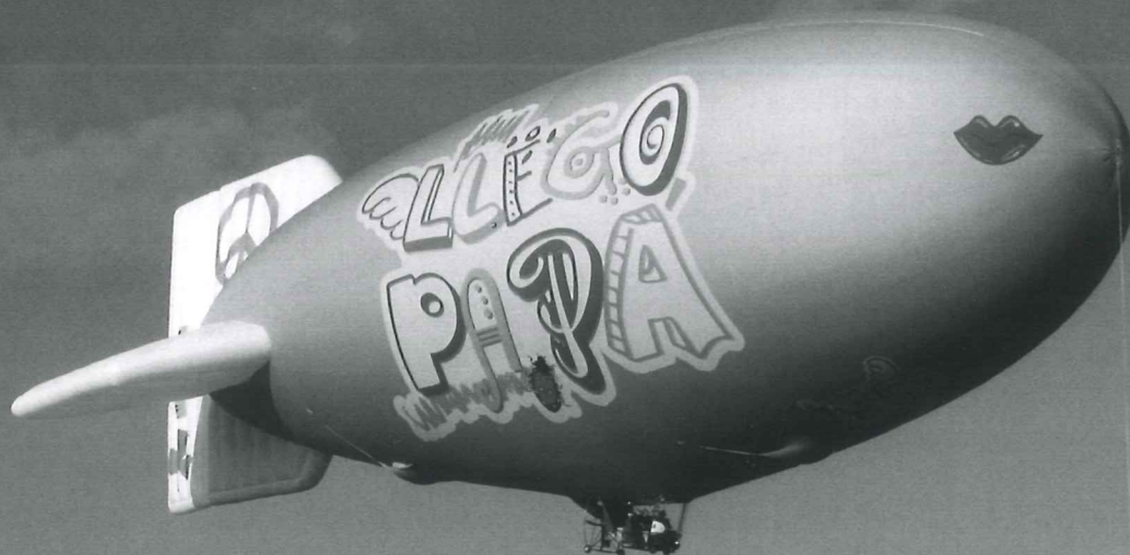
The GEFA-FLUG AS 1056 GD six seat hot-air airship.
