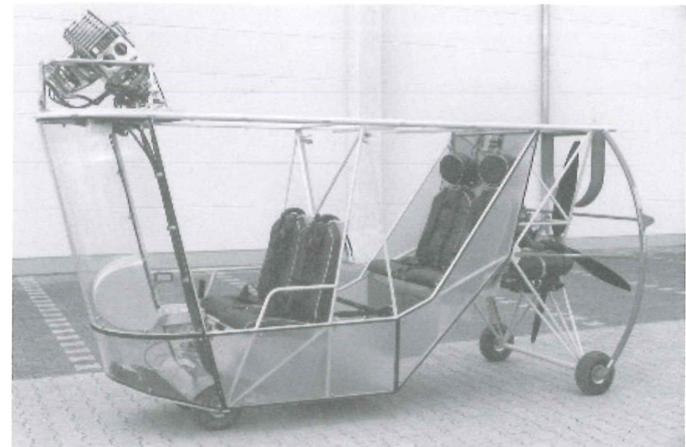
Figure 23.11. AS 105 GD four-seater gondola; the double burner unit is to be seen on the front top.
