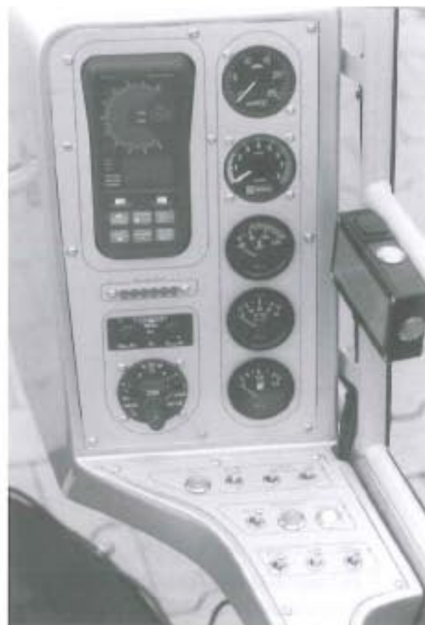
Figure 23.10. AS 105GD instruments and switch panel. The burner control unit can be seen to the right.
