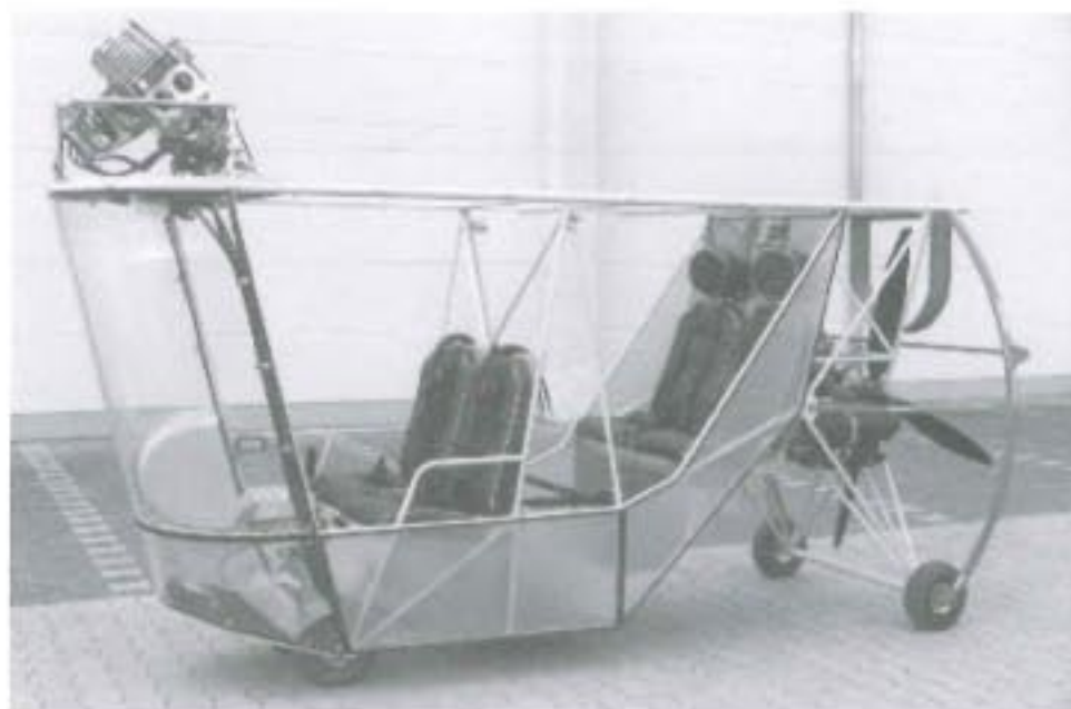
Figure 23.11. AS 105 GD four-seater gondola; the double burner unit is to be seen on the front top.
