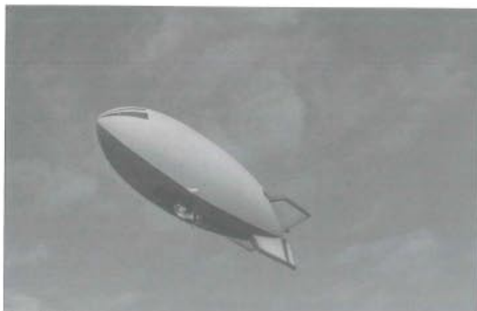
Figure 23.3. GEFA-FLUG no. 1 airship on its maiden flight in spring 1990. AS80GD uses a twin-seater Thunder & Colt gondola. The fineness ratio of the envelope has been increased to 3:1 to make these airships significantly slimmer and, therefore, faster.
